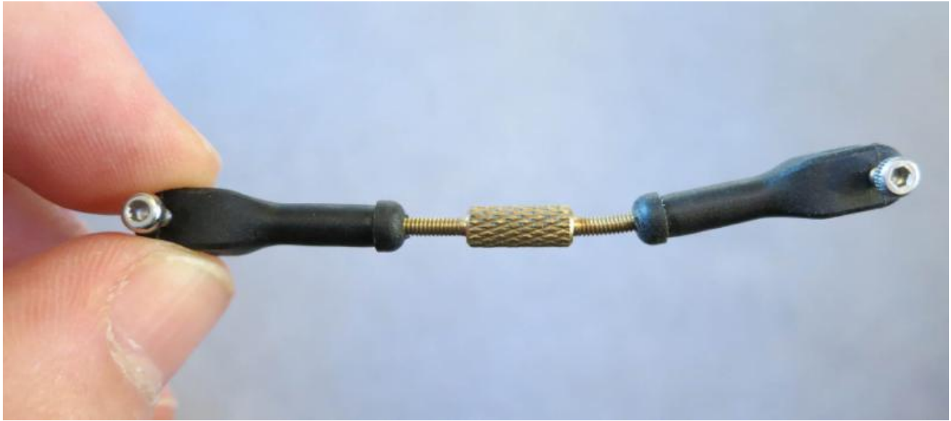
Photo 4 (Photo credit: John Tushingham) November 2012. A testing casualty. An early compression strut that clearly needed to be a lot stronger.
